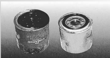
Clogging oil filter
